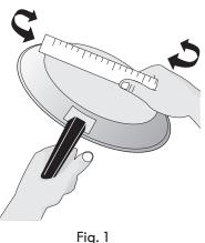
Check for flatness by rotating a ruler across the bottom of the cookware (See Fig. 1). Cookware should have flat bottoms that make good contact with the entire surface heating element (See Fig. 2). For more detailed information about the ceramic cooktop see Cooktop maintenance and Cooktop cleaning in the **Care & Cleaning** section.
